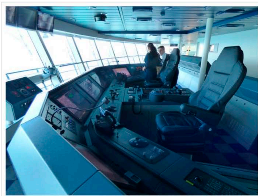
The horseshoe-shaped main bridge console.
