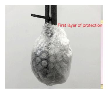
If the original shipping crate has been discarded and needs to be recreated, we recommend proper support for the housing, as seen in the following pictures. It is best practice to assign one person to manipulate the sphere and another to handle the housing. Use of cotton or latex gloves is a must to prevent damages and stains to any surfaces.
