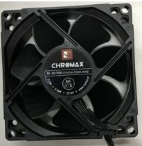
Present or not depending on the composer, a single or two fan(s) is(are) used to extract the warm air out of the housing, to prevent damages to the electronics. The fans are mounted to the housing part facing the ceiling, with rubber pegs to prevent vibration noises. To this day, the Noctua NF-A8 PWM has been used and liked. The Chromax NF-A8 PWM could be a good replacement unit, however, do consider the rubber pegs provided with the Noctua are the best to seat the fan onto the housing.
