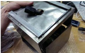
While lifting the top, managing power cabling through the housing hole, this would free the top or give you enough roomspace to rest the housing's top nearby while having a clear access to the inside of the housing.
