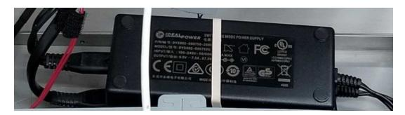
Power supply(ies) used in the housing may vary in amount. They feed the motherboards and the IR Remote receiving boards. The total wattage of a single sphere would vary from 75W to 300W. The used power supply, so far, is the Ideal Power 15DYS902-090750G.
