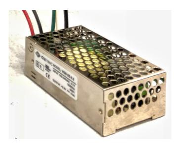
Power supply(ies) used in the housing may vary in amount and power, size and shape. They feed the motherboards and the IR Remote receiving boards. The total wattage of a single sphere would vary from 60W to 300W,
