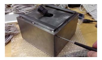
Lift the top part of the housing. Note that two sides of the box are attached to the back of the box and could grip electronic components in the move, pay attention to any restriction to avoid pulling connections out.
