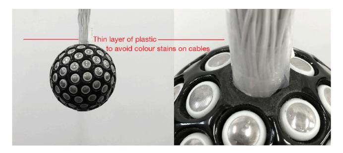
Then, the bundle should be tied (with a reusable tie-wrap preferably), about 10 centimeters away from the sphere. After, a pipe insulation sleeve (or any kind of protective foam) should be wrapped around the bundle to protect the cables.
