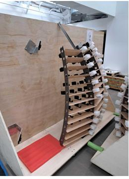
Next, gently place the slice on its back, ensuring it rests on the provided foam cubes. It is crucial to avoid applying additional weight to the part to prevent damage to other wooden slats.
