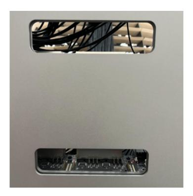
Finally, to clean the ethernet cables running between the sphere to the controllers, first use a vacuum cleaner to get the excess dust on the bundles. Then, you should use a compressed-gas duster to get in the spots the vacuum cannot reach.
