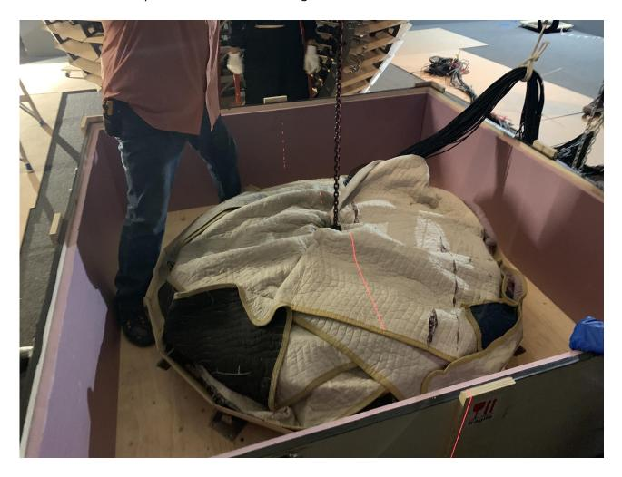
Lift up the dome using the blockchain, always have 1 person on each side keeping it in balance.
