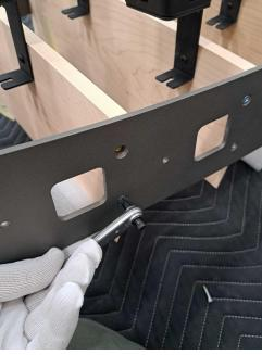
Each row of the sphere contains a different model of slat and each individual slats has unique speaker anchoring hole positions. Consequently, the provided spare slats do not have their brass inserts or holes premade.
