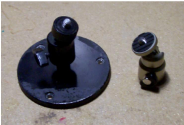
The one on the left is great since you can easily bolt it to anything. The one on the right is also good but it is a bit more difficult to mount since a bolt must come down into the swivel joint. This is actually just a \$10 tripod with the legs removed.
