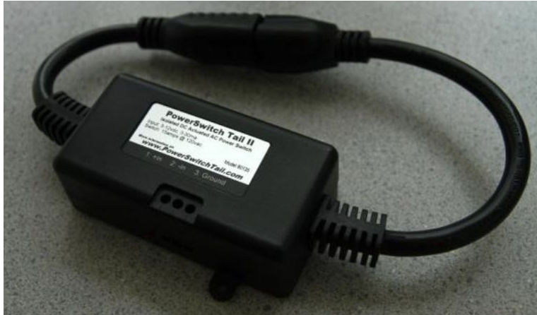
PowerSwitch Tail II Normally Open, AC relays to switch fans
