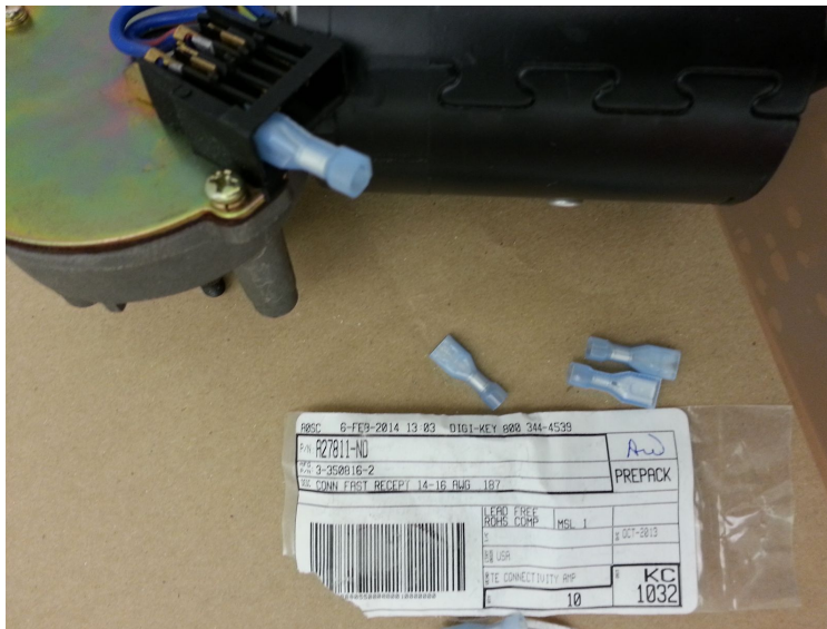
Motor DC connectors, 4.75mm Quick Connect Female 14-16 AWG (part # 3-350816-2)
